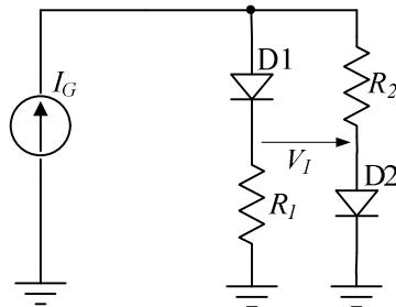
$$V_{D1} + R_1 I_{D1} = V_{D2} + R_2 I_{D2}$$
