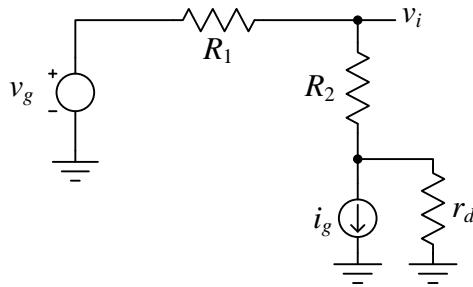
$$v_i = \frac{R_2 + r_d}{R_1 + R_2 + r_d} v_g - \frac{r_d}{R_1 + R_2 + r_d} R_1 i_g = 0.376 \text{ V} \sin \omega t,$$
