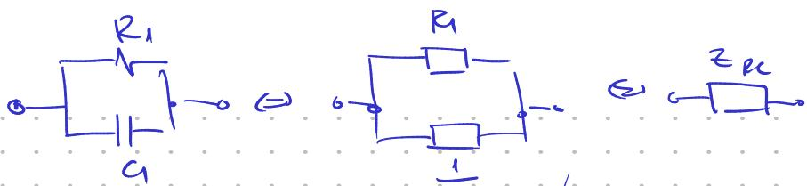
$$\begin{aligned} Z_{RC} &= R_1 \parallel \frac{1}{sC_1} = \frac{R}{sC_1} = \frac{R_1}{1 + sR_1C_1} \\ Z_C &= \frac{1}{sC_1} \\ V_{OP} &= \frac{1}{2}v_I - \frac{v_I}{2R_2} \cdot \frac{R_1}{1 + sR_1C_1} \\ &= \frac{V_I}{2} \left( 1 - \frac{R_1}{R_2} \frac{1}{1 + sR_1C_1} \right) = \frac{V_I}{2} \left( \frac{R_2(1 + sR_1C_1) - R_1}{R_2(1 + sR_1C_1)} \right) \end{aligned}$$
