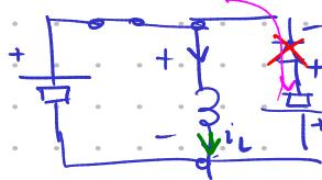
$$L \frac{di_L}{dt} = V_G - i_L R \Rightarrow \frac{di_L}{dt} = \frac{V_G}{L} - \frac{i_L}{L R} = \frac{10 \text{ V}}{100 \mu\text{H}} - \frac{1}{10 \mu\text{s}} = 100 \frac{\text{A}}{\mu\text{s}}$$
