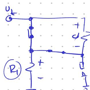
$$(P_{R1}^{DC}) = \frac{|V_z[0]|^2}{R_1} = \frac{(2 \text{ V})^2}{100 \Omega} = 4 \text{ W}$$
