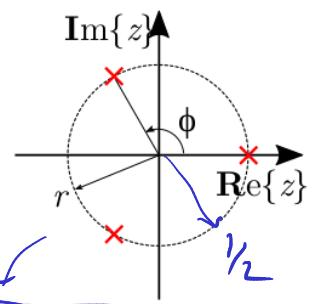
$$H(z) = \frac{H\phi}{(z-p_1)(z-p_2)(z-p_3)} \quad \left\{ \begin{array}{l} p_1 = r \\ p_2 = r e^{j\phi} \\ p_3 = r e^{-j\phi} \end{array} \right.$$
