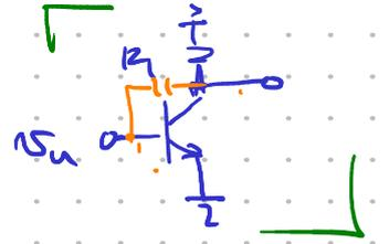
$$v_I = v_U \cdot \frac{R_1}{R_1 + \frac{1}{sC}} - G_m v_U \cdot \frac{\frac{1}{sC} \cdot R_1}{\frac{1}{sC} + R_1} = v_U \frac{sCR_1}{1 + sCR_1} - G_m v_U \cdot \frac{R_1}{1 + sCR_1} \Rightarrow$$
