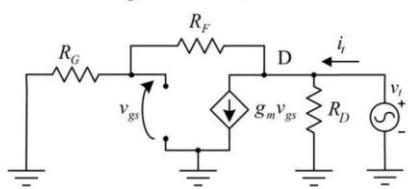
$$i_t = g_m v_{gs} + \frac{v_t}{R_F + R_G} + \frac{v_t}{R_D}$$
