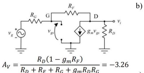
$$A_V = \frac{R_D(1 - g_m R_F)}{R_D + R_F + R_G + g_m R_D R_G} = -3.26$$
